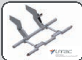
Hydraulic foldable bumper suited for GVW >= 8T
