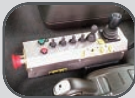
Electro-pneumatic cab controls
