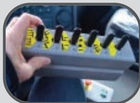
Pneumatic cab controls
