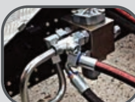
Hydraulic lines for double circuit
