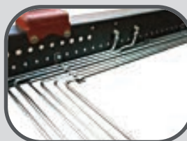
Tubing for rear accessories Under run, axle blocking or stabilizer roller
