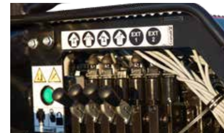
Support leg valve Electrically/manually operated. 4-6-8 sections adapted to 1-circuit, 2-circuit and LS systems.
