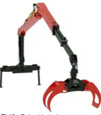
**TL12** • Robust L-design cranes, newly updated with next generation technology and modern solutions. Available in single or double telescope versions and with alternative reaches. The TL-crane can be laid extended at the top of the load for an effective and rapid move to the next work site.
