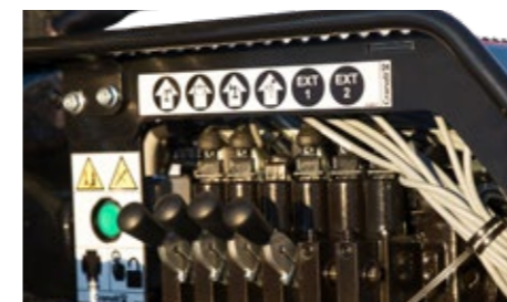
Support leg valve Electrically/manually operated. 4 sections suitable for single-circuit, dual-circuit and LS systems.
